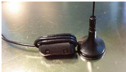
SWR of the stock whip with a 11.5cm radius ground plane.
